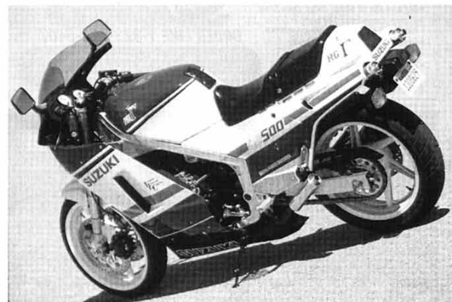
An immaculate example of the average modified Gamma would be Barry Adam's '86 RG500. Besides the Wolf pipes, Adam also retrofitted a Honda CBR600F3 front rim and a CBR-F2 rear rim, to allow the use of the latest radial rubber.
