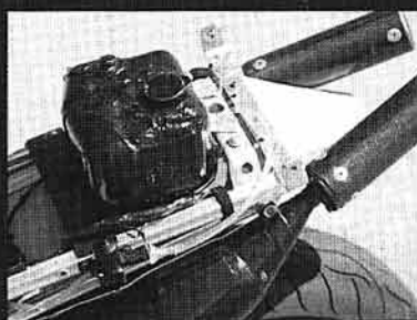
Removing the rear tail section reveals the reservoir for Norian's trick water-injection system. By injecting water into the exhaust and cooling the expelling gases, the system fools the pipe into thinking it's a different length, boosting midrange horsepower.
