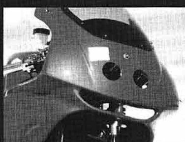
The front fairing was originally meant for a Kawasaki ZX-6R, but it fits up well. Norian was going to fill in the ram-air ducts, but he decided to leave them in to complete the happy-face look.
