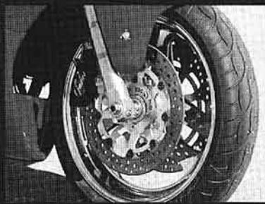
A Lindemann-revalved 1990 GSX-R fork graces the front end, with GSX-R calipers biting on EBC ProLite discs. The front wheel is a 3.5 x 17-inch Performance Machine unit, shod with the ubiquitous Dunlop D207 GP radial.
