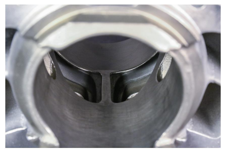
Notice the chamferred edges of the ports. This is critical to prevent 2-stroke piston ring/locating pin failure. Need tips for your cylinder? <u>Read our complete guide to cylinder prep here.</u>
