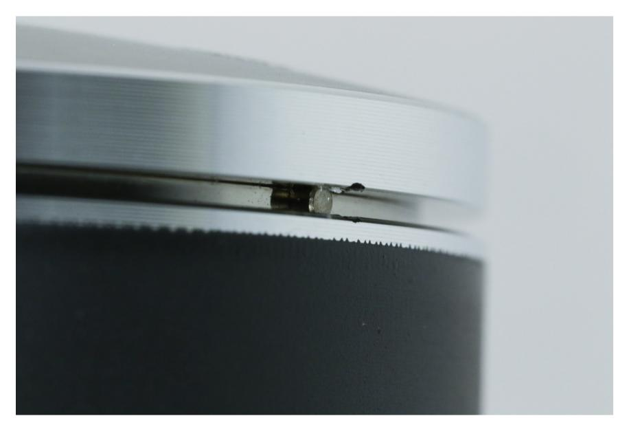
2-stroke pistons have a very small feature that is unique to 2-strokes only: the locating pin. Here, Wiseco takes an in-depth look at what a locating pin is, what its function is, and why 4-strokes don't need it.
