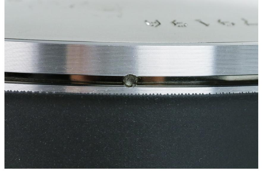
Locating pins must be made from high-strength material.
