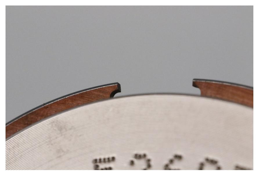
Especially in high-performance 2-stroke engines, it's important to have strong material that resists wear from heat stress. This is why all Wiseco 2-stroke pistons are forged. You don't want that ring end gap spinning and causing complete engine failure.
