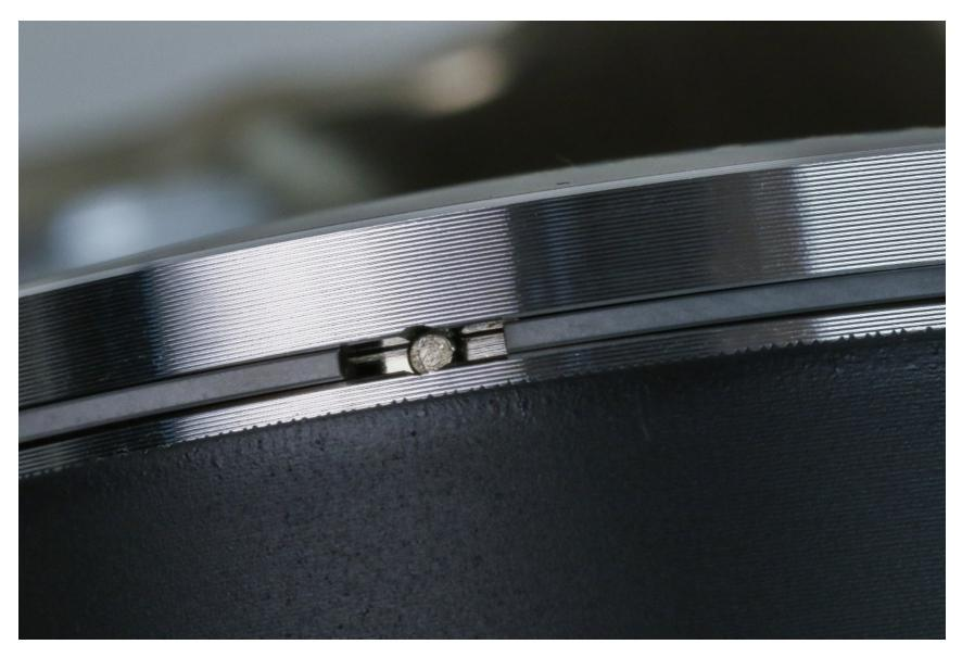
If the piston ring expands while passing over a port, it can put excess stress on the locating pin, potentially breaking it and leading to catastrophic failure.
