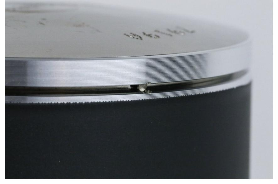
Locating pins are inserted using an interference fit, so machined dimensions on both the piston and the pin are critical.
