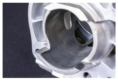
"The locating pin's job is to keep the end of ports in the cylinder wall. If the ring end gap the ring from moving so that it does not end up in an opening or a port hole," explains Dave Sulecki, Global Powersports
